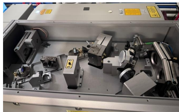
Ti:Sa laser installed
